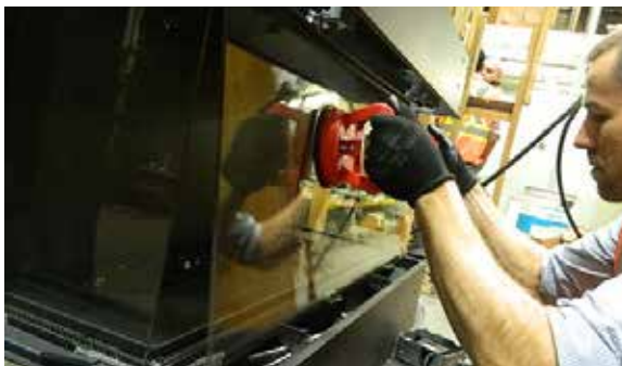
Handle front panel with supplied vacuum clamps
